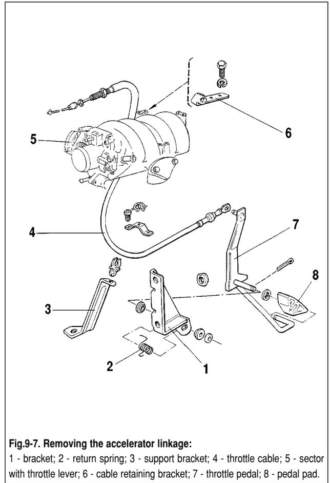
**Fig.9-7. Removing the accelerator linkage:**
