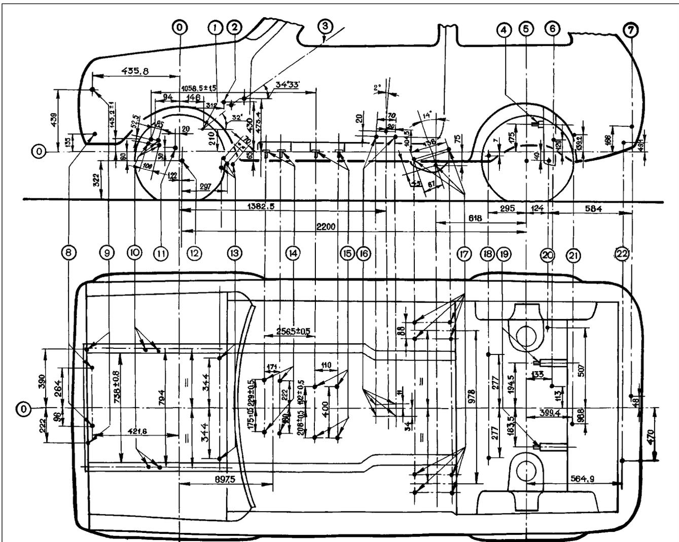
Fig.8-4. Anchorages of vehicle units and assemblies:
