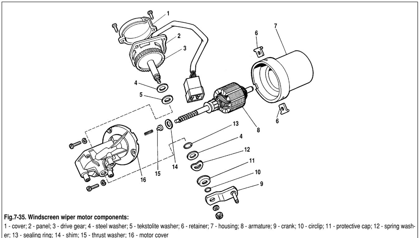
Fig.7-35. Windscreen wiper motor components:
