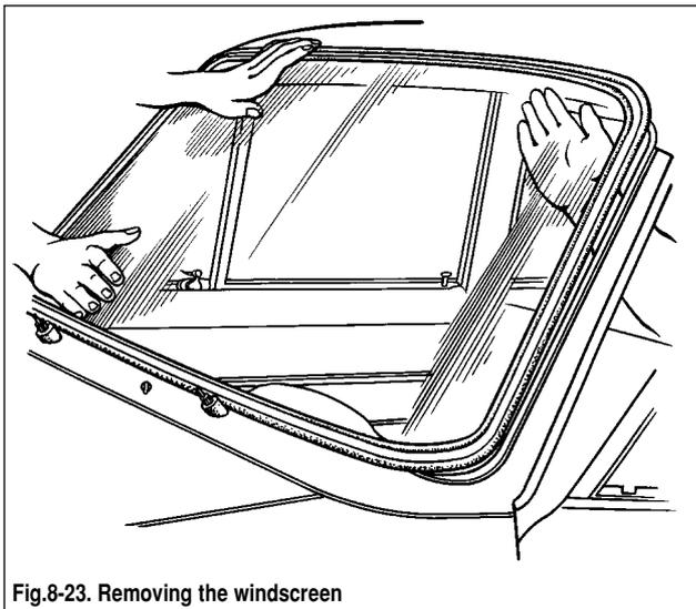
Fig.8-23. Removing the windscreen
