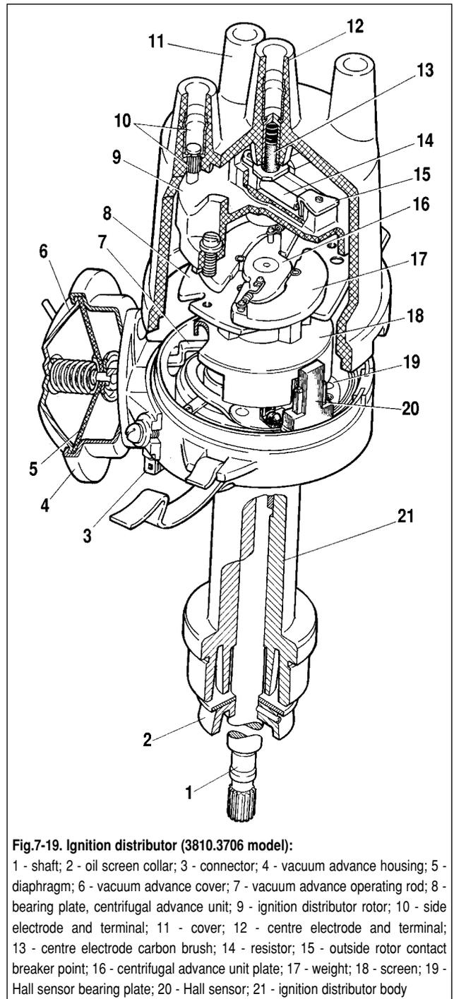
Fig.7-19. Ignition distributor (3810.3706 model):
