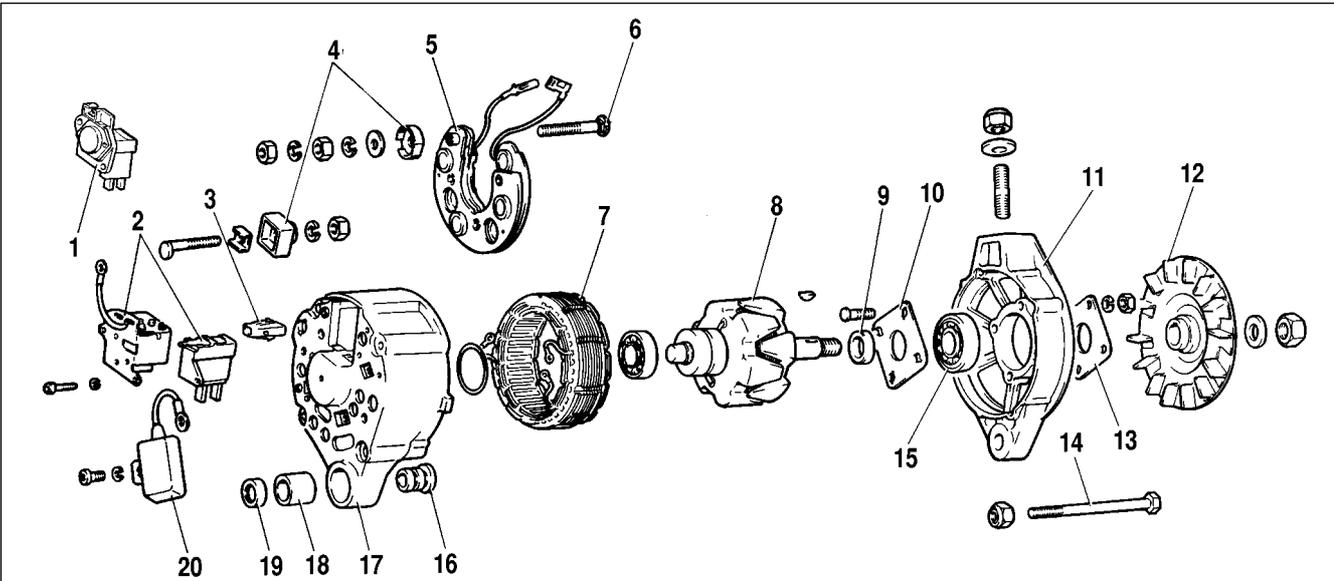
**Fig.7-12. Alternator components:**
