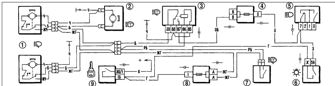
Fig.7-36. Wiring diagram for headlight wipe/wash:
