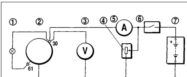
**Fig.7-5. Wiring connections for diode plate test:**
