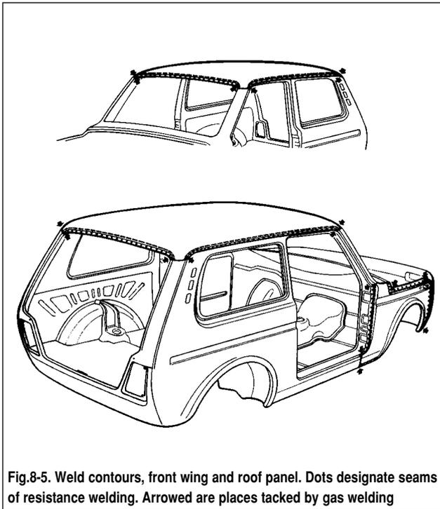
**Fig.8-5. Weld contours, front wing and roof panel. Dots designate seams of resistance welding. Arrowed are places tacked by gas welding**
