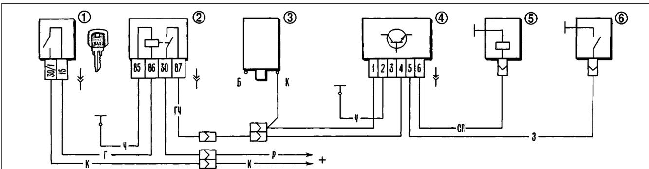
**Fig.7-41. Fuel cutoff solenoid control system wiring diagram:**
