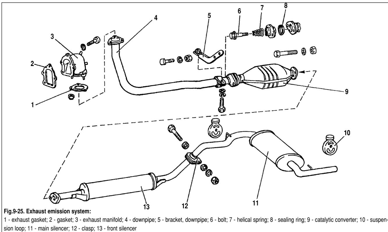
**Fig.9-25. Exhaust emission system:**
