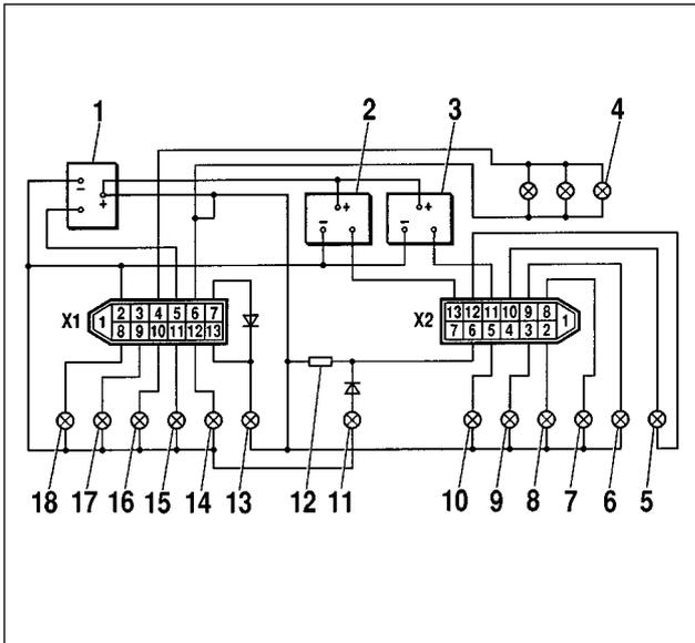
**Fig.9-36. Wiring diagram for instrument cluster:**
