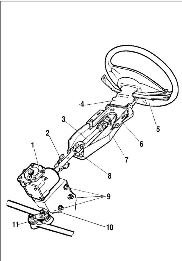
**Fig.9-37. Steering components:**
