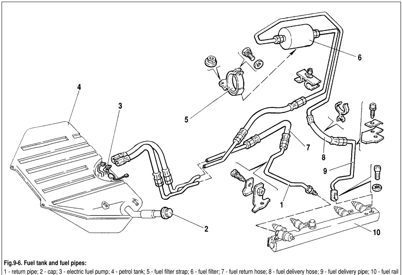
**Fig.9-6. Fuel tank and fuel pipes:**
