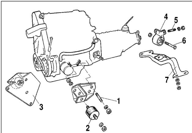
**Fig.9-19. Engine support:**
