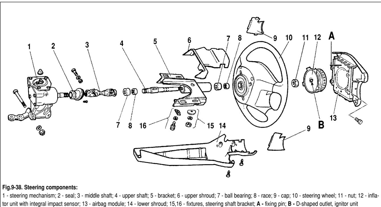
**Fig.9-38. Steering components:**
