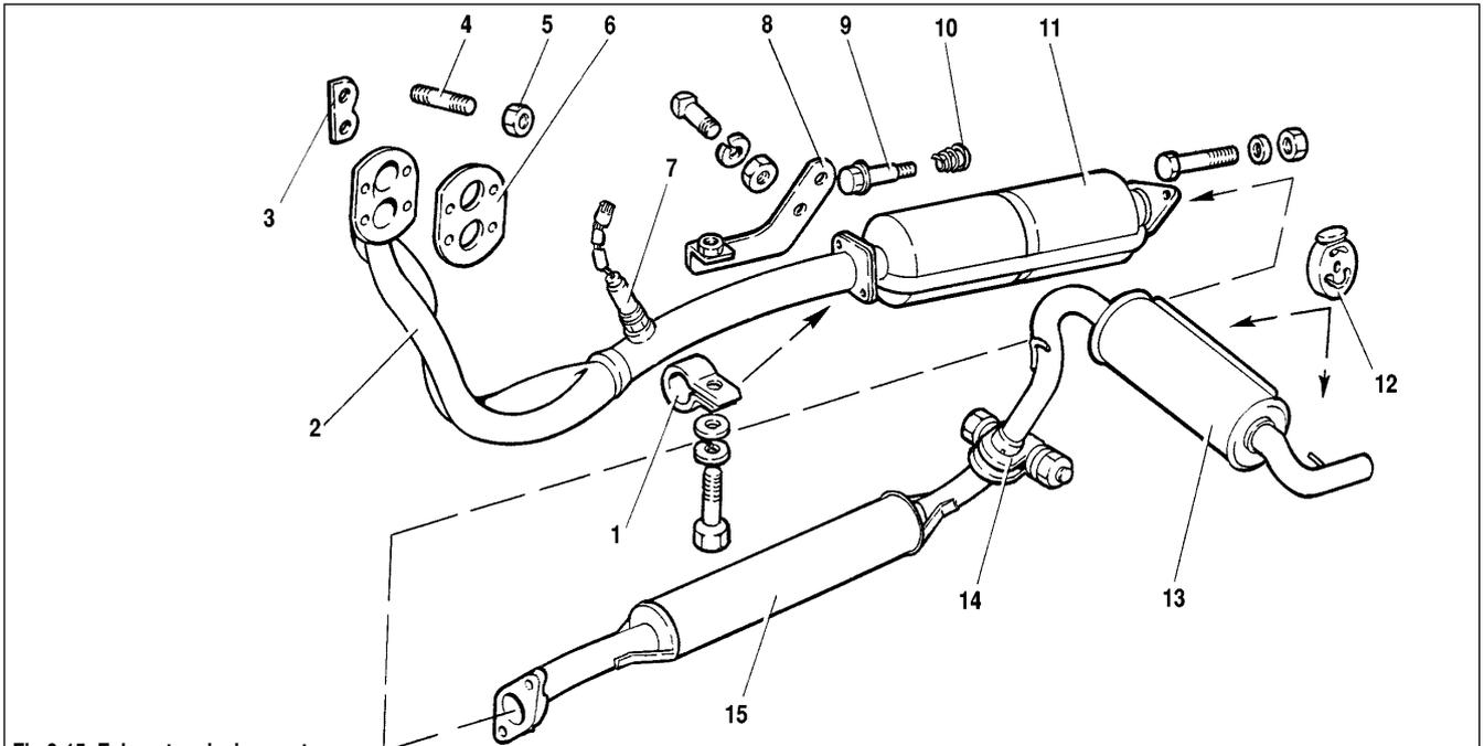
**Fig.9-15. Exhaust emission system:**
