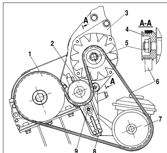
**Fig.9-23. Removing and refitting the alternator drive belt:**
