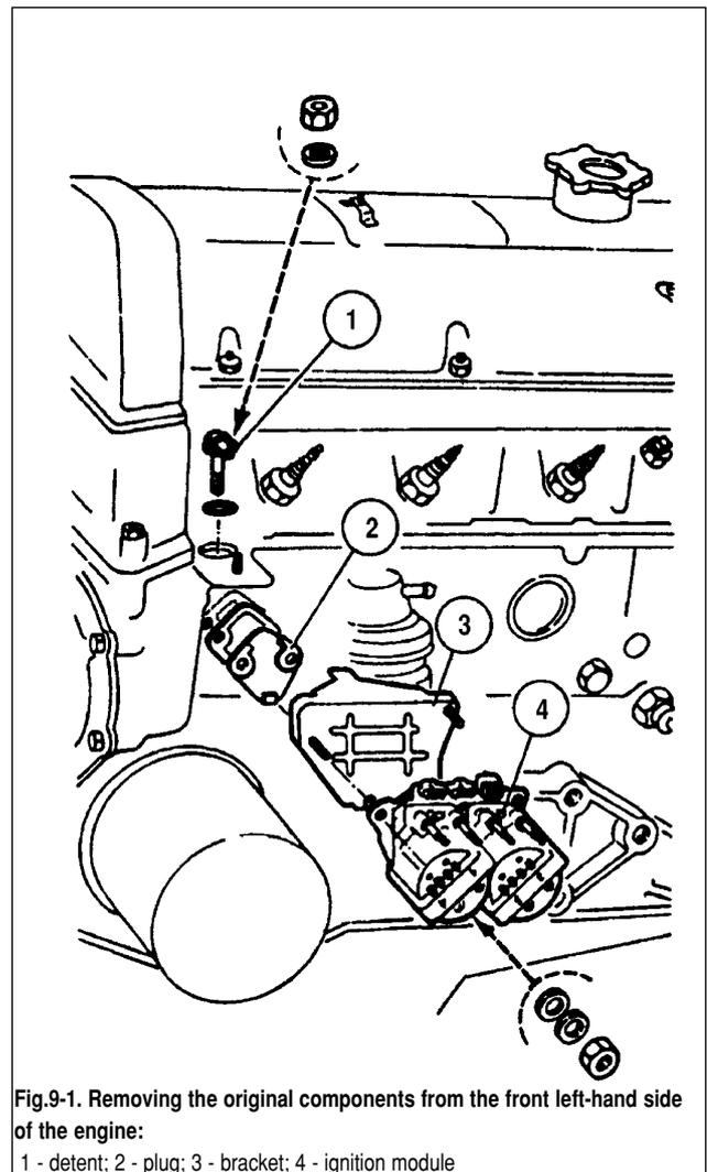
Fig.9-1. Removing the original components from the front left-hand side of the engine:
