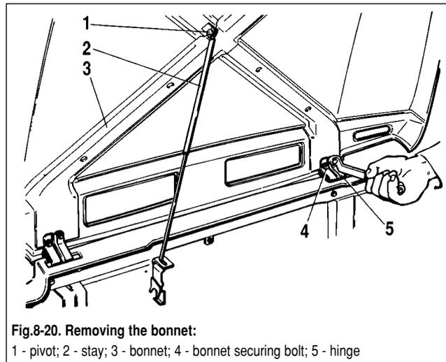
Fig.8-20. Removing the bonnet:
