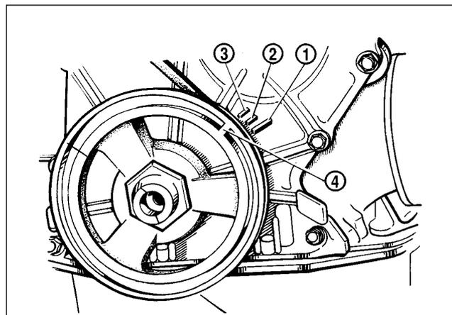
Fig.7-18. Ignition timing marks:
