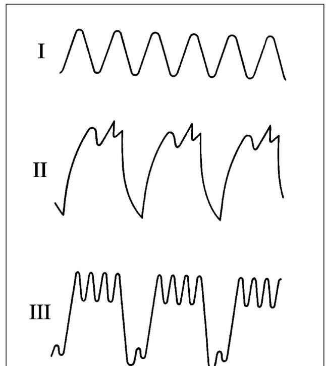
**Fig.7-7. Alternator rectified waveform:**
