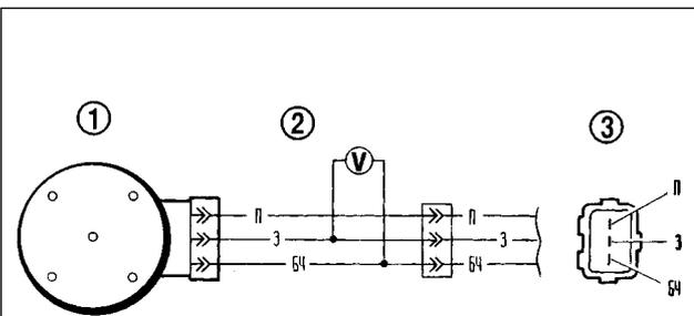
**Fig.7-23. Wiring diagram for Hall sensor in-vehicle test:**
