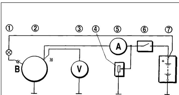
**Fig.7-6. Alternator wiring connections for oscilloscope test:**
