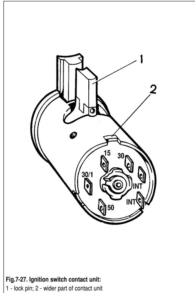
Fig.7-27. Ignition switch contact unit:
