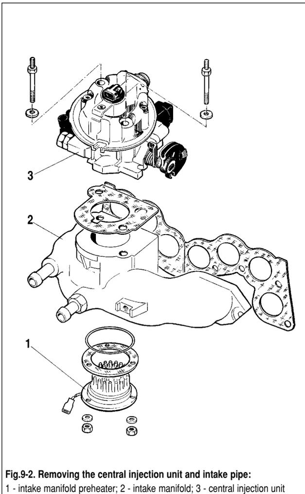
Fig.9-2. Removing the central injection unit and intake pipe:
