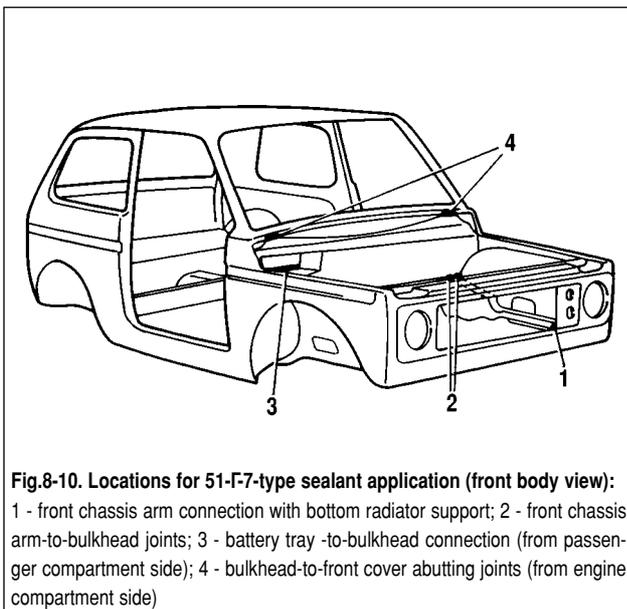
**Fig.8-10. Locations for 51-F-7-type sealant application (front body view):**
