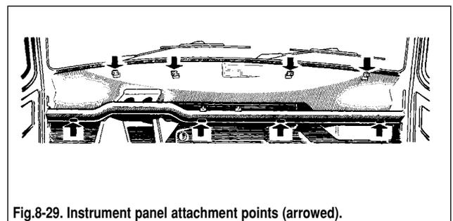
**Fig.8-29. Instrument panel attachment points (arrowed).**
