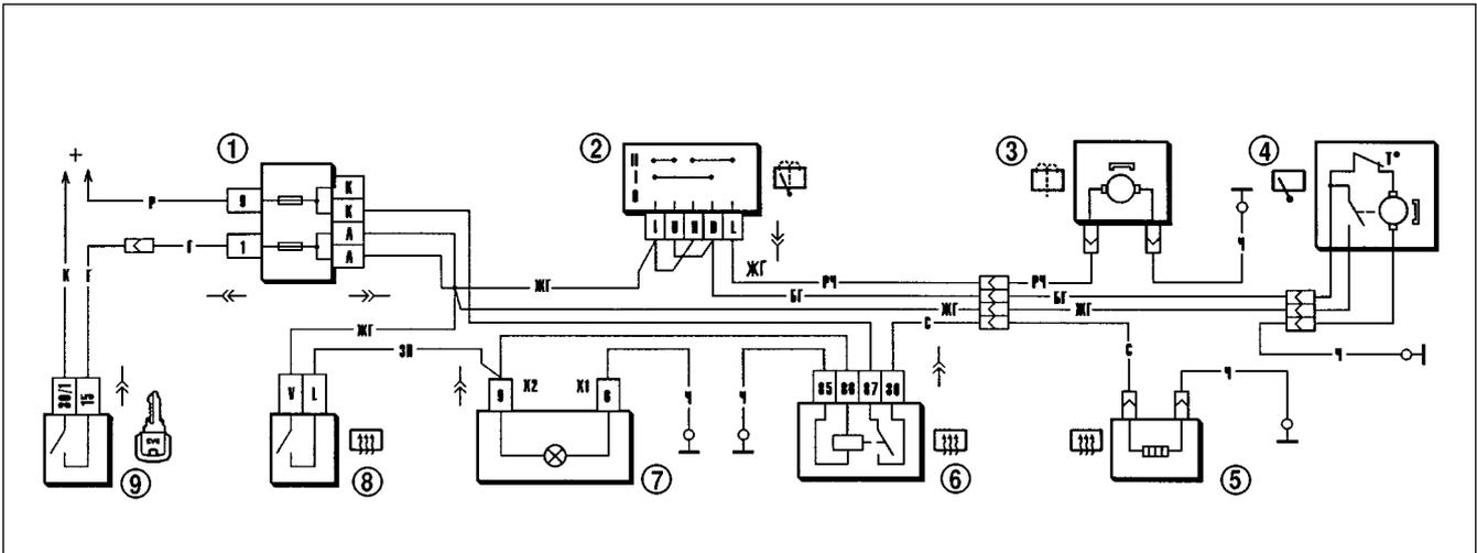
**Fig.9-33. Wiring diagram for tailgate wipe/wash and heating element:**
