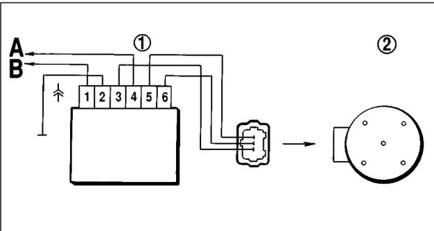
**Fig.7-20. Checking the ignition distributor on the test bench:**
