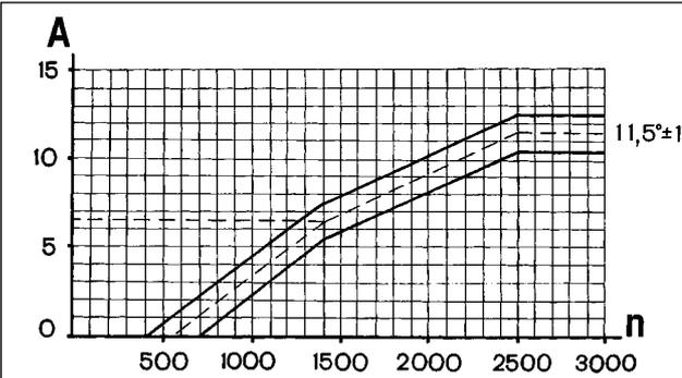
**Fig.7-21. Centrifugal advance ignition distributor map:**
