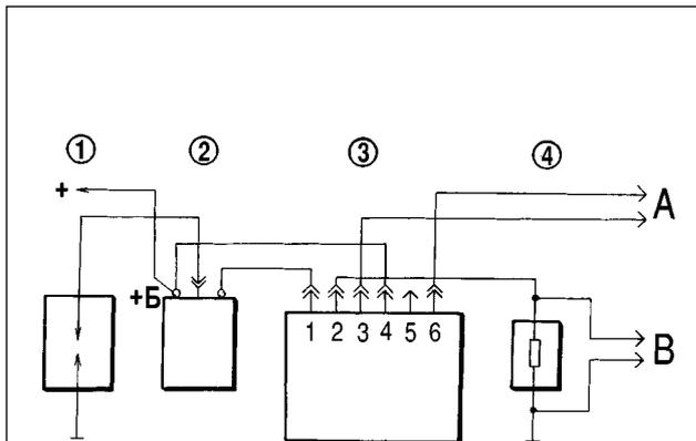
**Fig.7-25. Checking the spark control module:**
