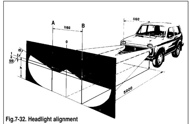
Fig.7-32. Headlight alignment
