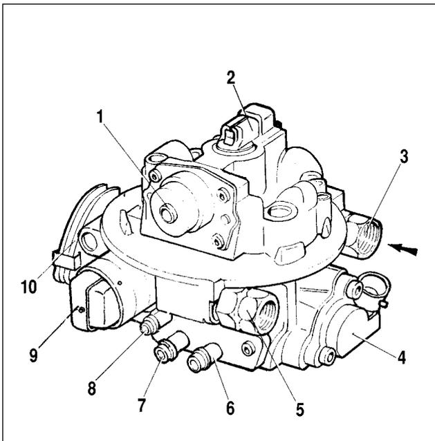
**Fig.9-3. Central injection unit:**
