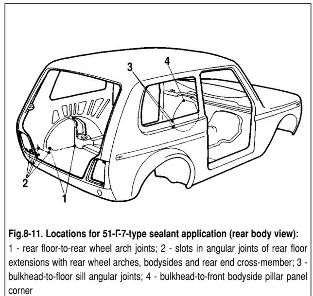
**Fig.8-11. Locations for 51-F-7-type sealant application (rear body view):**
